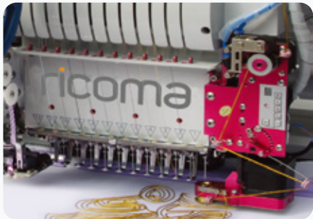
Cording Device (CD-E) Easily create an embroidery effect with the cording device, which lays a cord of fabric and attaches the cord with transparent zigzag stitches.
